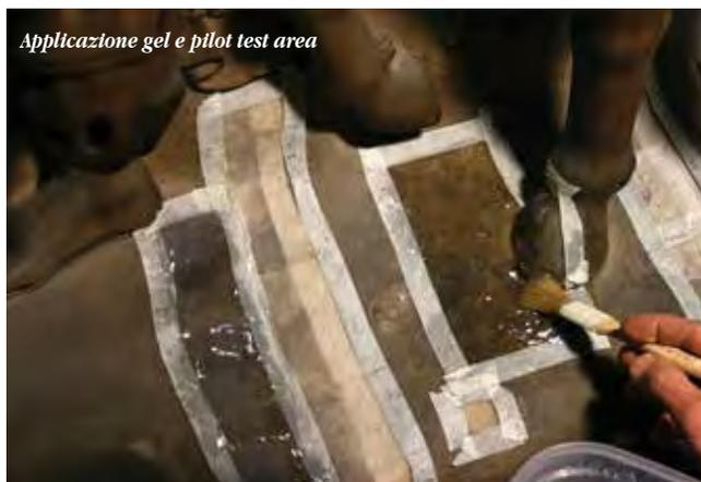
*Applicazione gel e pilot test area*
